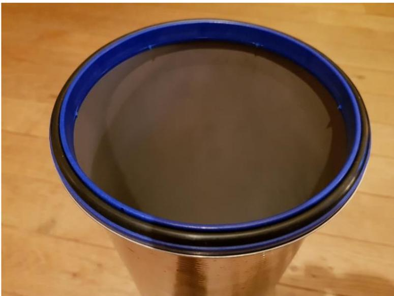
Properly place (stable = horizontally flat) the O-ring on the lower edge of the Biofilter stainless steel housing
