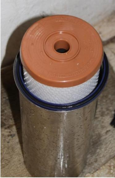
Check that the **2 O-Rings** (2 black rubber gaskets coiled on either side, above and below the blue plastic ring, intended to guarantee the tightness of the filter) are present
