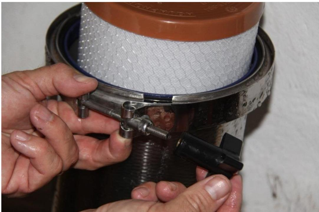
**Make sure that the stainless-steel strapping slide of the Biofilter matches the contours of the housing of the filter as shown in the photos below:**
