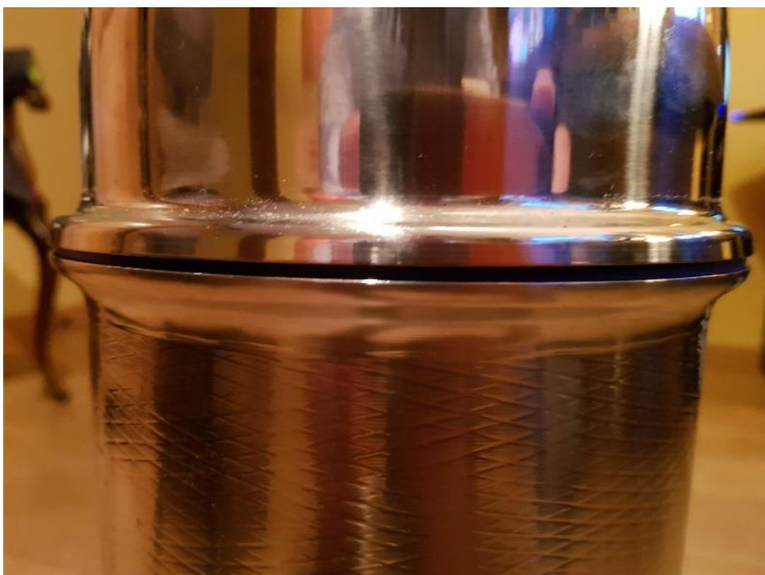
Close the filter using the black knob, screwing the ring tightens the strapping slide to seal hermetically the filter. There remains a small free space in the middle of the strapping slide (the 2 parts of the strapping slide do not touch!), picture below.
