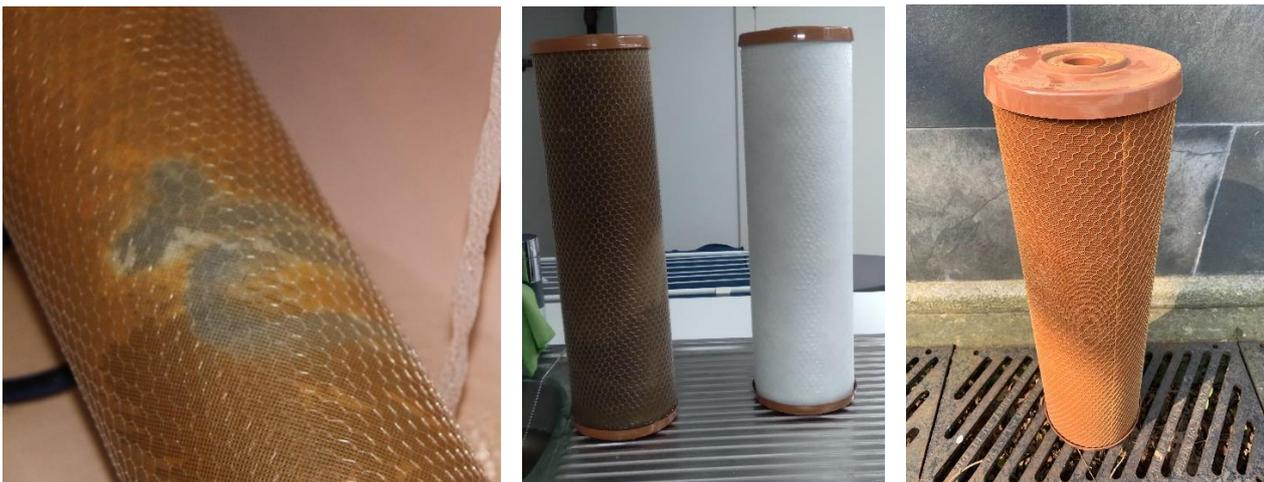
*Photo of the rust saturating a non-replaced cartridge (due to the galvanization of the pipes of the water supply company)*
